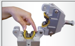
The die snaps quickly into the press fixture requiring no pins or screws.
