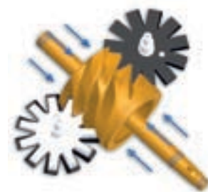
Axial loads act on both sides of the main rotor.
