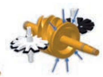
Radial loads act on both the top and underside of the main rotor.
